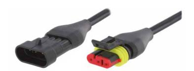
Number of contacts:2–6Wire gauge:0.34–2.5 mm²Rated voltage:24 V AC/DC, more on requestDegree of protection:IP67 in mated condition
